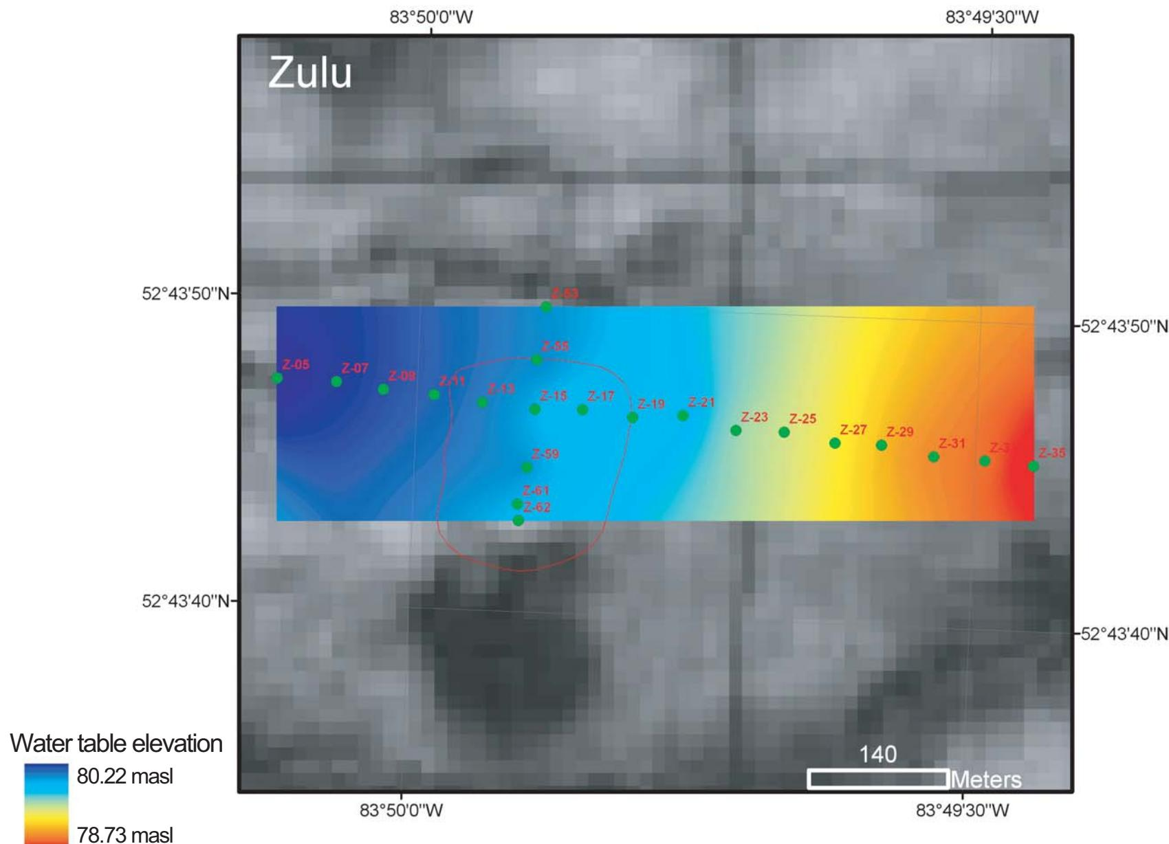
Figure A-2. Peat groundwater flow direction at Zulu based on kriging of water table data.
